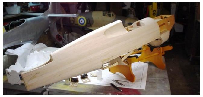
From this photo you can see the 12mm stabiliser mounts are fitted and the rudder and tail wheel steering pull-pull cables have been threaded through the fuselage before the planking is closed up.
