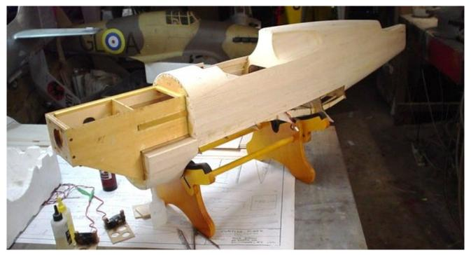
The picture above shows the planking is now complete down to the wing fillets. The fillets require the wing to be fitted and then the final planking can be done down to join up with the ply sheet in the wing cut outs. A good, no gap fit results, I hope!
