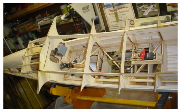
Its easier to fit some of the hardware while the plane is still a skeleton. In the pictures above and following you can see the air tank behind the head rest, the tail wheel retracting servo mounted on the angled former, the high torque elevator servo mounted in a box epoxied to the spruce frame and the angled former and the pull pull rudder and tail wheel steering servo mounted on the forward frame. The elevators and tail wheel retract will be actuated by a carbon fibre tube pushrods.
