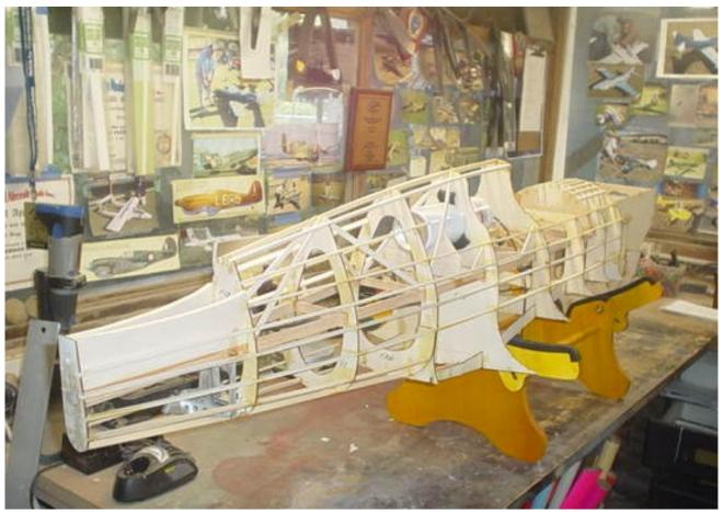
With the unfortunate experience of having to add a lot of lead weight to the nose of the Hurricane to get it to balance correctly I was extremely mindful of any weight aft of the C of G while I was building the Kittyhawk. All the stringers are balsa and the only real weight will be the spruce crutch, the carbon tube pushrods for the elevator and tail-wheel retract actuation and the tail wheel retract assembly itself.
